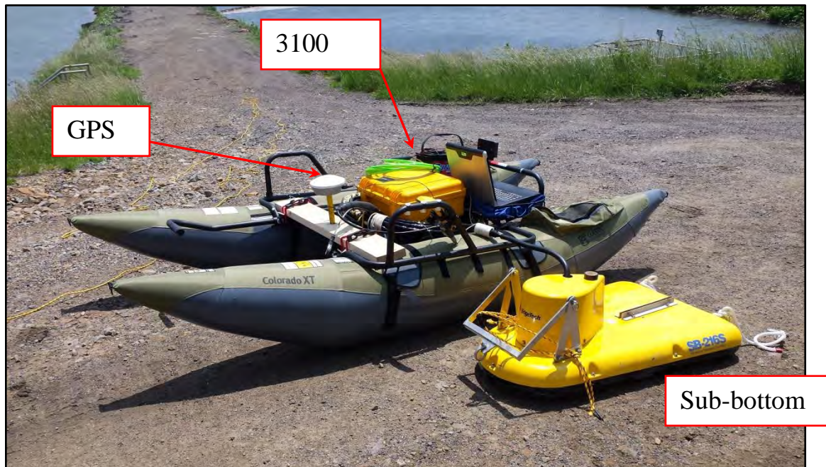
Picture Showing the GPS, 3100 Topside Unit and 216 Sub-bottom Unit (towfish)
